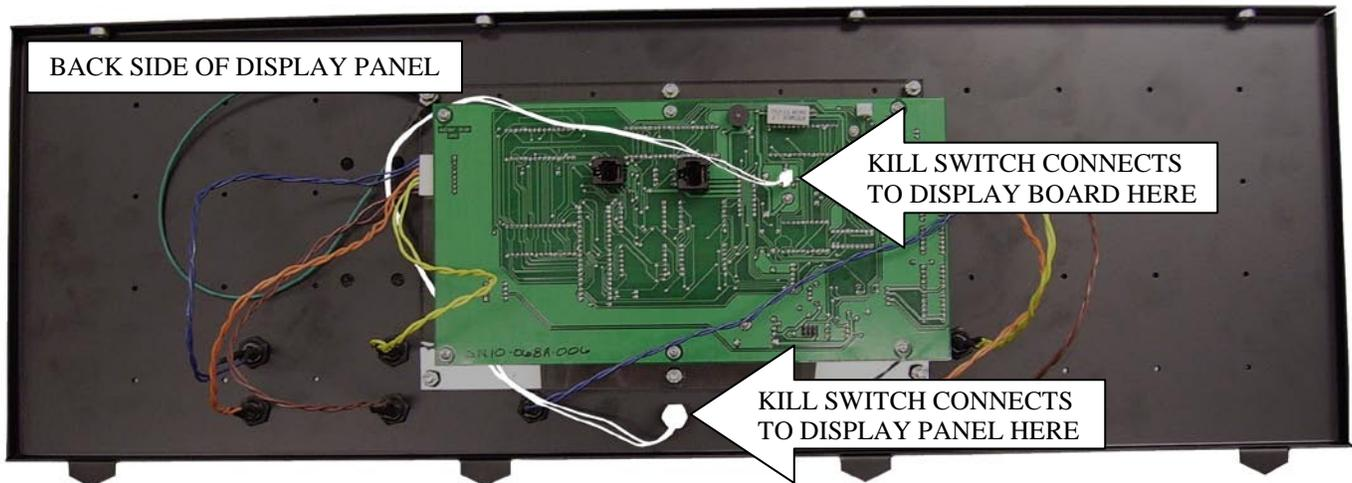
Older display boards will appear slightly different, but the magnetic kill switch will connect in the same locations. The magnetic kill switch in this picture has been made white for better visibility.
