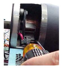
Slide the brush back in place in the top part of the slot, and hold in place while re-inserting the clip.
