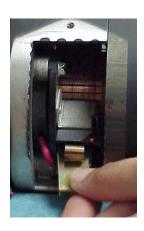
Pull the brush out of the slot and check the size. If the longest side is less than ¾ inch long, replace both brushes in the motor.
